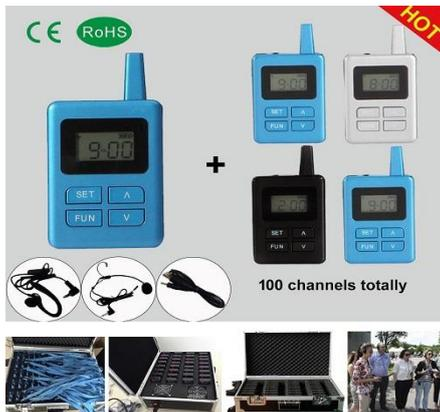
5. If the Guide need adjust the “channel”, customers just press “FUN” and “V” together, then you can see “ch” twinkles, then just press “A” or “V” to select the channel which you like. Just make sure the channel is same as Transmitter and Receiver. (Use step is same as Transmitter and Receiver.)
